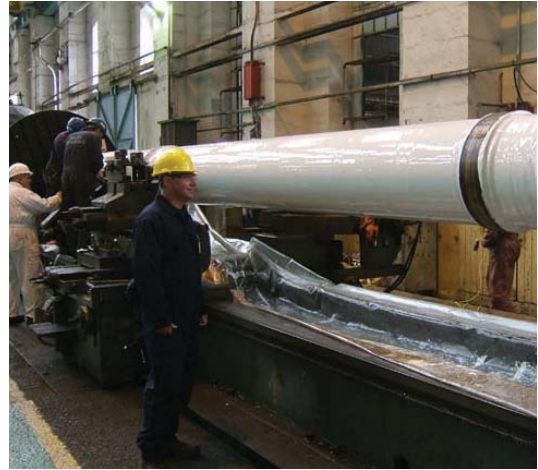
Shaft is coated with Thor-Coat corrosion free coating and anti-fouling coating
