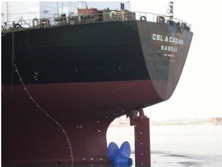
CSL Acadian converted to seawater lubricated COMPAC from oil in 2006
