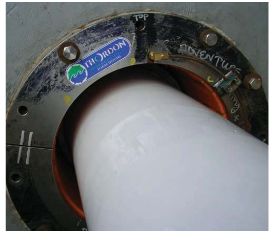
When refitting shaft, care is taken to protect shaft coating from damage from chains, etc.
