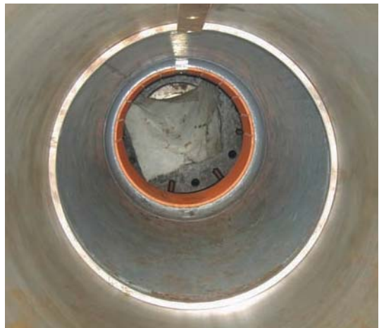
Stern tube housing is coated with anti-corrosion paint
