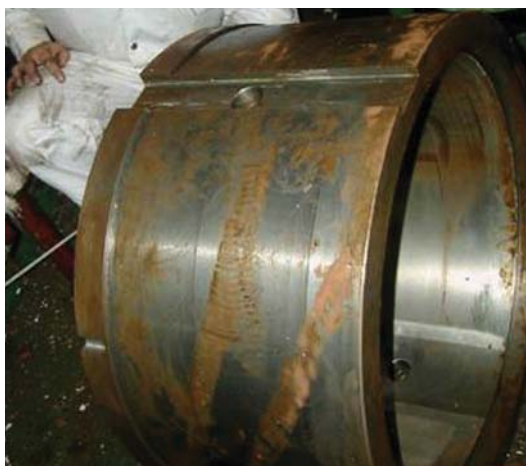
Remove the original white metal bearings
