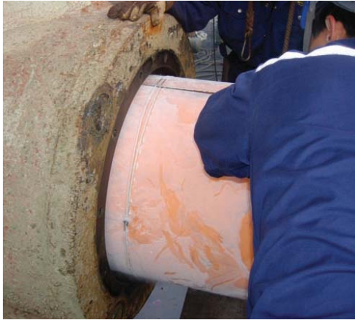
Bearing is cooled in liquid nitrogen and fitted into stern tube
