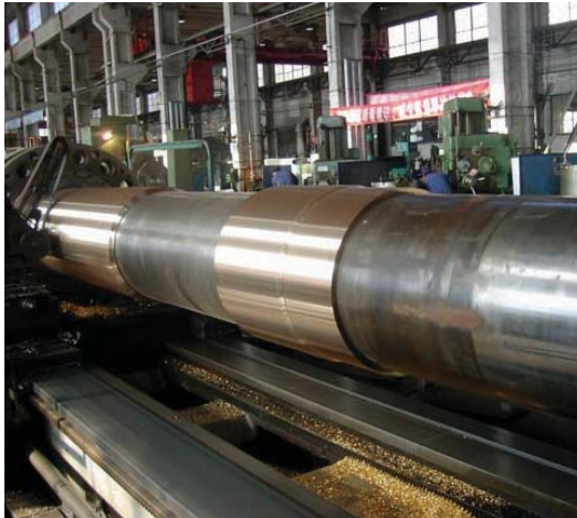
Shaft liners are machined on lathe
